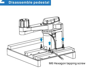
1. Use a adjustable wrench to remove the fixing screw.
